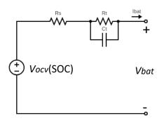
**Figure 3.** Thevenin-Based electrical model for a Li-Ion cell, with a series resistor  $R_s$ , an RC network ( $R_t$ ,  $C_t$ ) to describe basic charge transfer phenomenon, and an open circuit voltage dependent on the SOC  $V_{OCV}$  [9].
