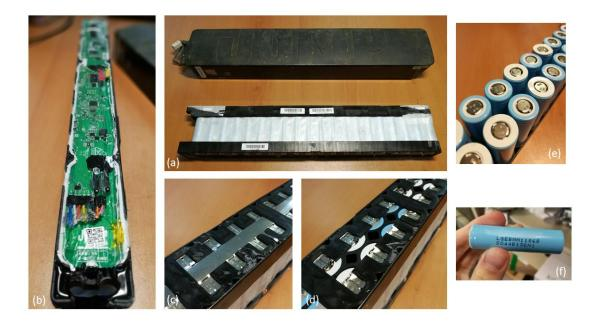
**Figure 2.** Example of the disassembly of an e-bike 10S4P Li-Ion battery. a) E-bike battery case and pack; b) BMS; c) d) Detail of a nickel strip before and after its removal, respectively; e) Cells without nickel contacts and the plastic support; f) Detail of a LG MH1 18650 Li-Ion cell.
