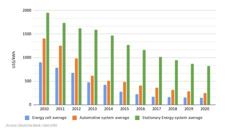
**Figure 1.** Evolution of Li-Ion battery cell and system costs for EV and stationary storage application [6].
