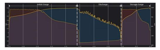
Figure 4. Voltage [blue] - Current [red] plot during a capacity-test. The cell-under-test is a LG MH1 of 3.200 mAh, tested by a MegaCellCharger charger.
